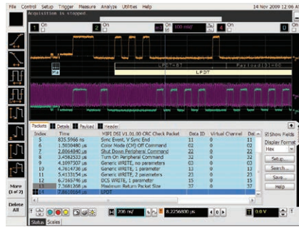
Trigger on and decode MIPI packets.
