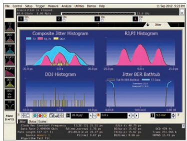
Analyze jitter plus RJ/DJ separation.
